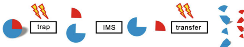
Fig. 1.11 A schematic diagram of CID experiments with ion mobility separation using SYNAPT
